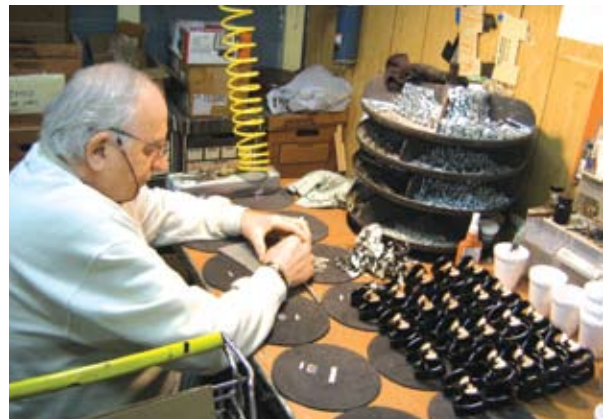
figure 9. Leon Marzani working on Westinghouse Type OB meter brake magnets (photo courtesy of Arcman Corporation).
